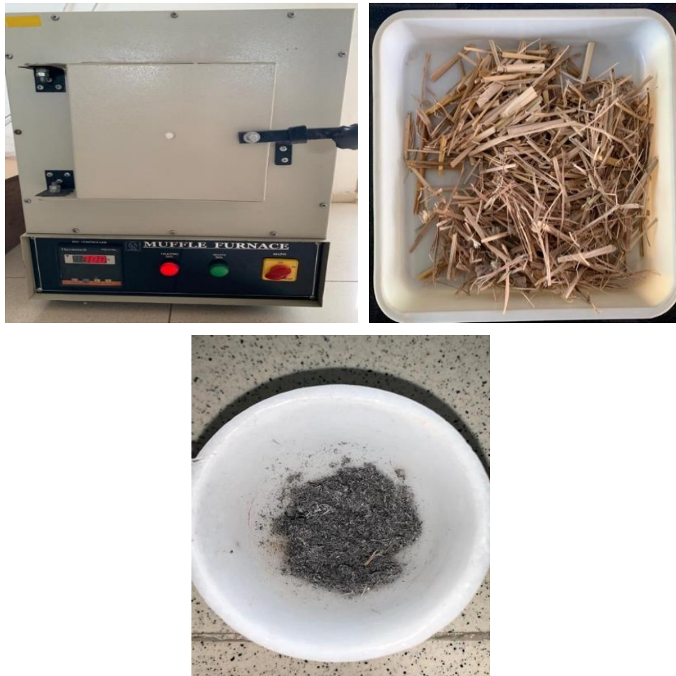
Figure 2: From left to right, muffle furnace set at 700 °C, the dried rice straw (RS) sample and the rice straw ash (RSA).
